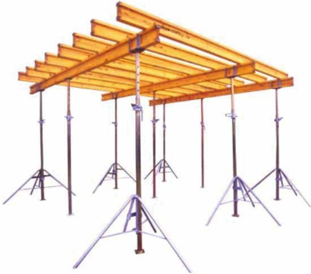
As a standard type, outer pipes are made of  $\text{Ø}60 \times 2.50$  mm, inner pipes  $\text{Ø}48 \times 3.00$  mm TSE certified pipes. The pipe wall thickness is the same in all sections of pipes. The mechanism is  $\text{Ø}60 \times 4.00$  mm. Nut is CE certified material and ductile iron. The system consists of adjustable strut and four-way head, Uhead, three legs, H20 header and under-beam headers, according to the H20 or 10x10 to be used.
