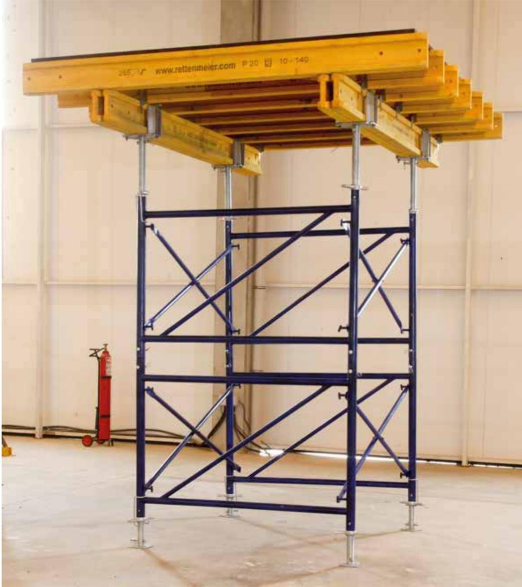
It is a scaffolding system with high carrying capacity. Load bearing scaffolding system gives you "SPEED, ECONOMY and CONFIDENCE". In order to ensure the stability of H frames, diagonal components produced in different lengths can be used to create any width of carrier scaffold. Each vertical pipe of the main frames can carry a load of up to 55 kN. Two different applications can be made with the H type load frame system.
