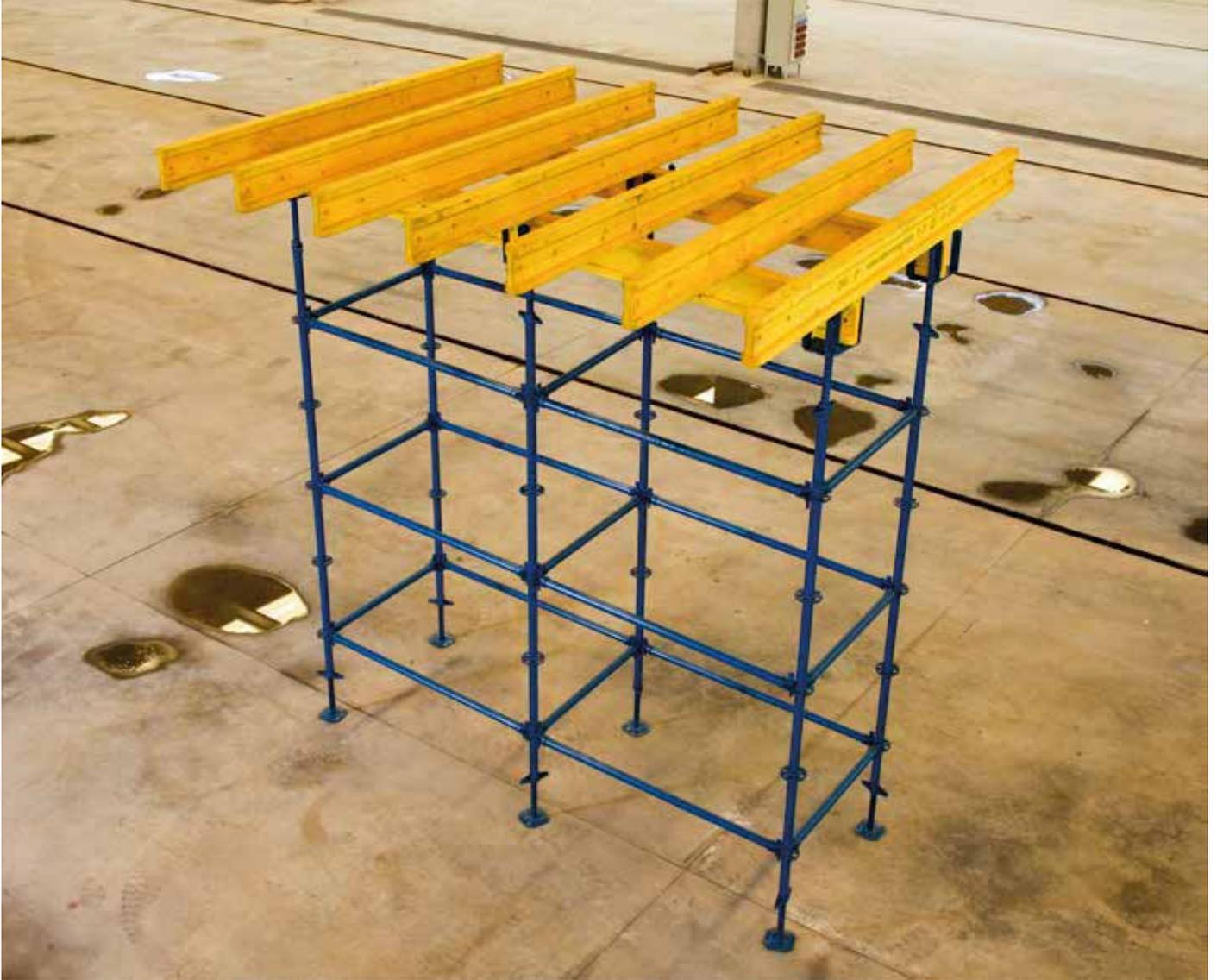
You can easily use flanged scaffolding system with slabs and beams. The carrying capacity can be up to 6 tons for each prop. Economical solutions can be obtained in high concrete thicknesses. The props that make up the system are produced from  $\text{Ø}48.3 \times 3.00$  mm TSE certified pipes. Flanges are 8 mm thick and A1 quality sheet metal is used. Welding is done by automatic arc robots. Connection can be made from 8 points on a single surface.
